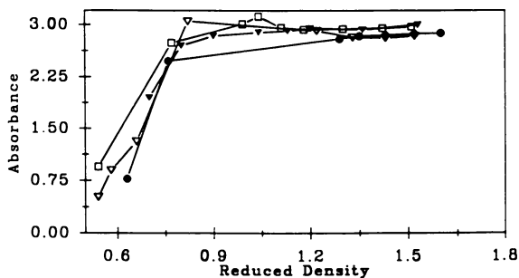
Figure 5. Steady-state absorbance (at 326 nm) for a sample that contains 100 \mu\text{M} pyrene as a function of \text{CO}_2 density. (symbol, T_r ): ( \bullet , 1.00); ( \nabla , 1.01); ( \blacktriangledown , 1.02); ( \square , 1.05).
